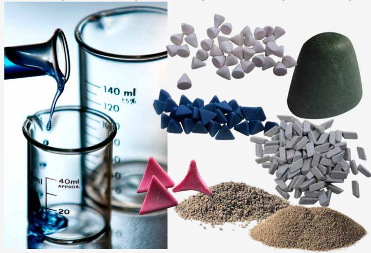
A brasives, Additives and Compound for processing in vibratory finishing equipment
